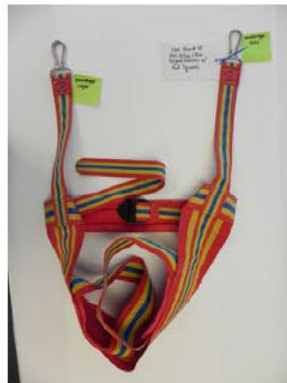
Figure 32 - Harness 42 needed 2 new clip straps.
