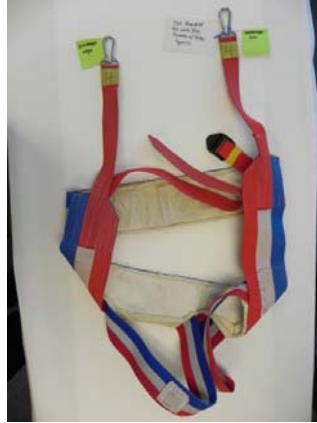
Figure 33 - Harness 44 needed new pads and clip straps.
