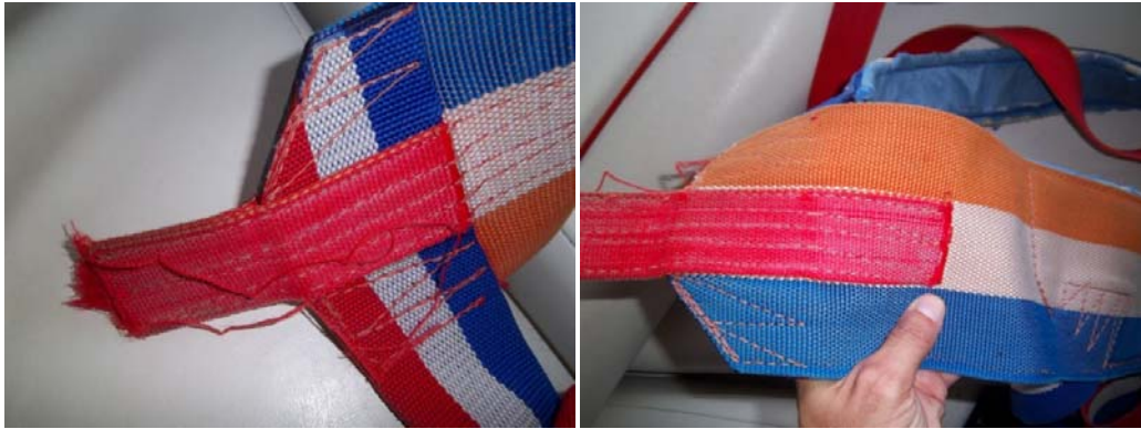
Figure 25 - Inside and outside portions of the hook risers where they connect to the seat strap.
