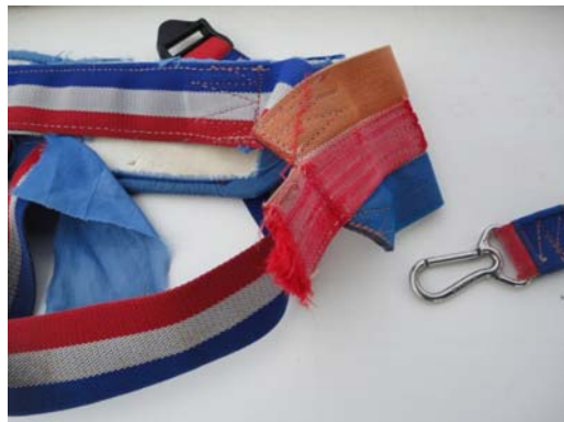
Figure 20 - Victim's harness showing failed strap (wearer's left side).
