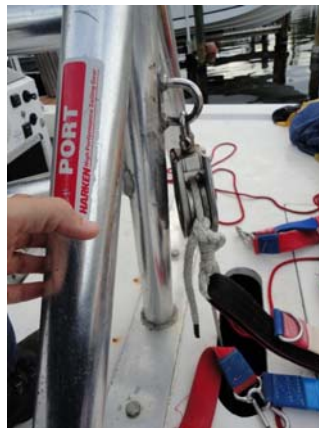
Figure 17 - Towline connection to yoke was a bowline with multiple half-hitches.
