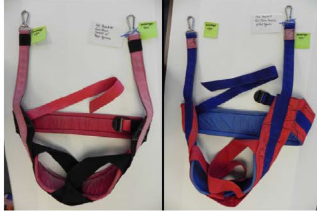
Figure 31 - Harnesses 40 and 41 were serviceable.
