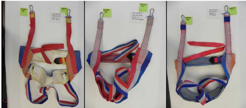
Figure 29 - Harnesses 37, 39 and 43 were not suitable for service.
