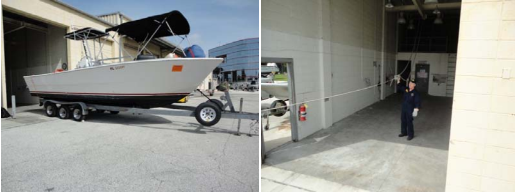
Figure 22 - FL0238 removed from evidence bay for winch test, and the configuration of the test equipment.
