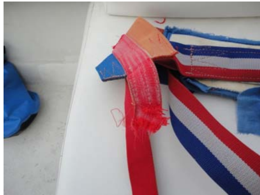
Figure 19 - Victim's harness showing failed strap (wearer's right side).
