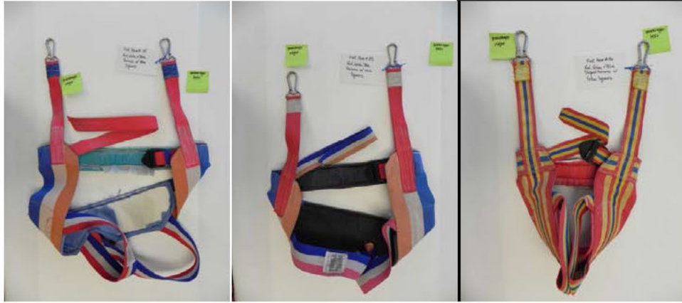
Figure 28 - Harnesses 34, 35 and 36 were not suitable for service.
